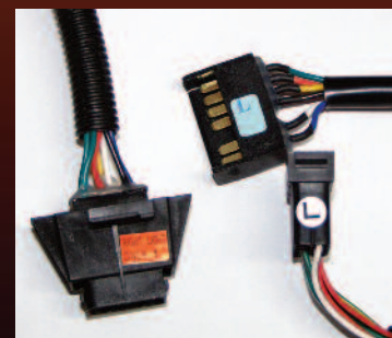
Wiring looms will usually be marked to show which side they go on
