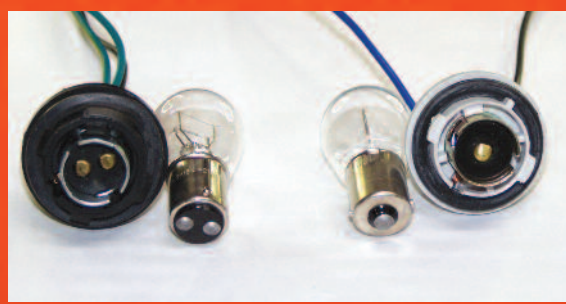
Two into one doesn't go - make sure the correct bulbs are fitted to the appropriate sockets
